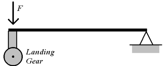
Figure 10: Static testing apparatus used to determine landing gear strength.
