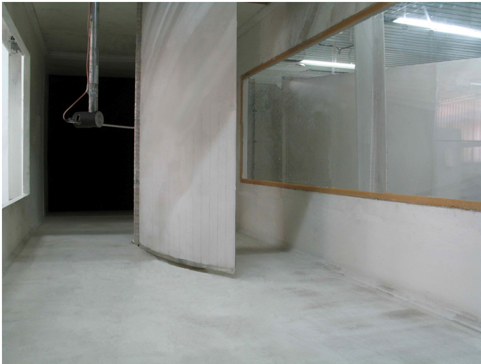
Fig. 4. Photograph of NLF-0414 airfoil model with ice shape in the test section.
