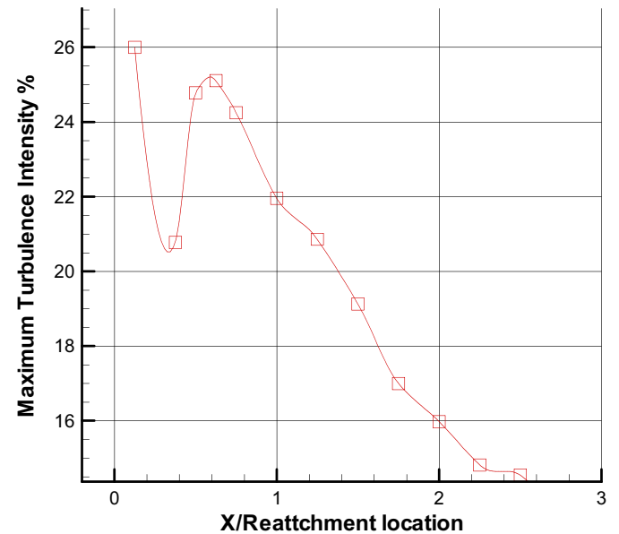
Fig. 17. Chordwise distribution of maximum streamwise turbulence intensity ( Re = 0.5 \times 10^6 , \alpha = 0 ).
