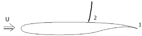
Fig. 6. Whitcomb supercritical airfoil. Flow from left to right. U is the free stream velocity. 2 indicates the separation region behind the shock.
