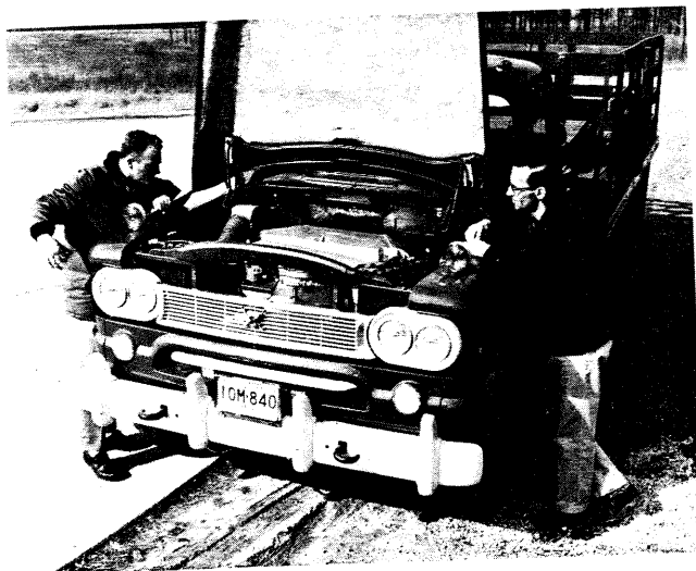
Fig. 16 - Third Turbine - Truck Installation
