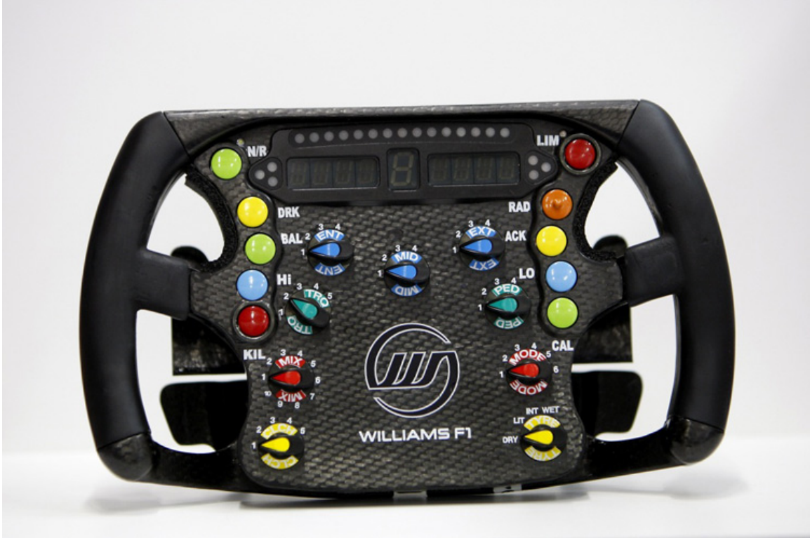
Rotary position switches are a fact of life in Formula 1...Fuel, suspension, traction control, braking bias and whatever the rules allow these days with the spec ecus from McLaren Electronics are all switchable on the carbon fiber steering wheel.
