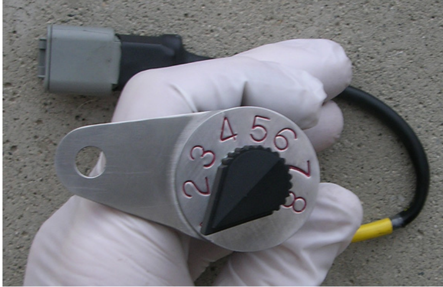
Eight Position Traction Control Rotary Switch. Seven resistors set voltages from 5 VDC to 0 VDC in equal steps.
