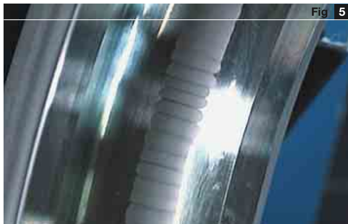
Fluting or washboarding in a raceway caused by electrical erosion
