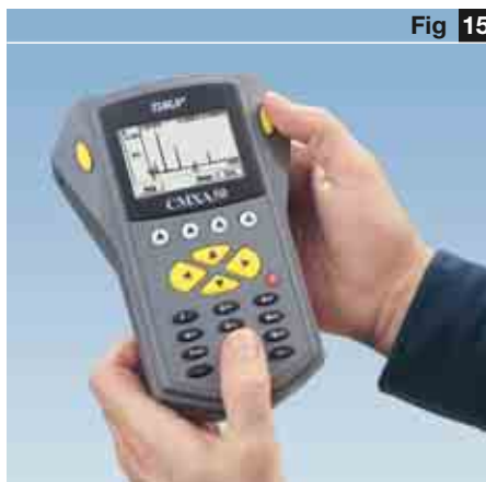
Vibration levels can be checked with SKF condition monitoring equipment
