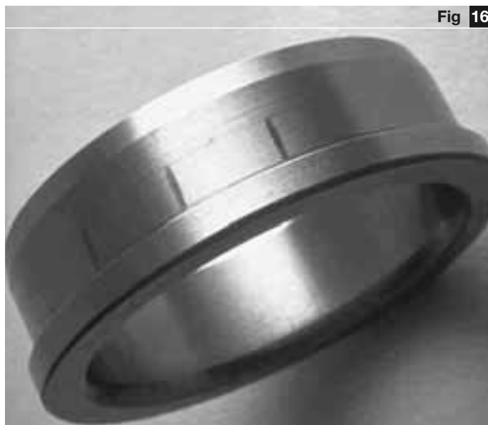
Transverse smear streaks from faulty assembly
