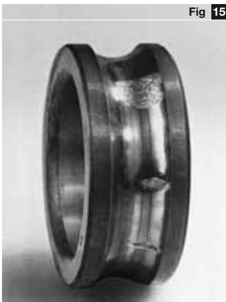
Mounting error: Flaking will start from the indentations at rolling element distance
