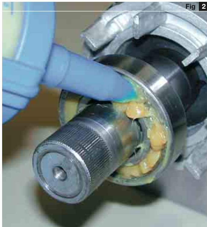
Greasing a deep groove ball bearing mounted on a rotor shaft
