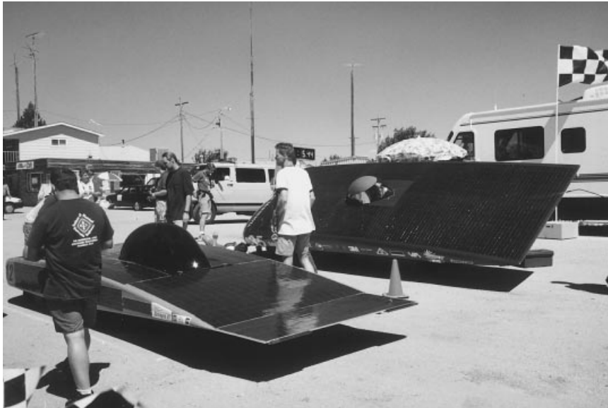
Figure 2. Solar arrays tilted for charging at the end of a race day and at a midday stop. In the top photo, the car in the foreground is the third-place finisher, from Stanford University. In the bottom photo, the car in the foreground is the fourth-place finisher, from Texas A&M University
