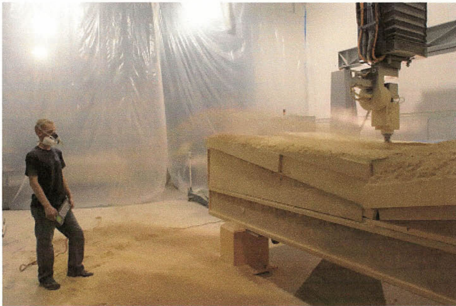
Figure 9: Borealis 3 Top Mold Rough Machining at PaR Systems
