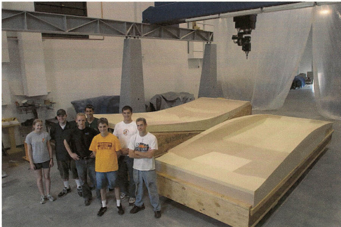
Figure 18: Borealis 3 Top and Bottom Molds after Machining
