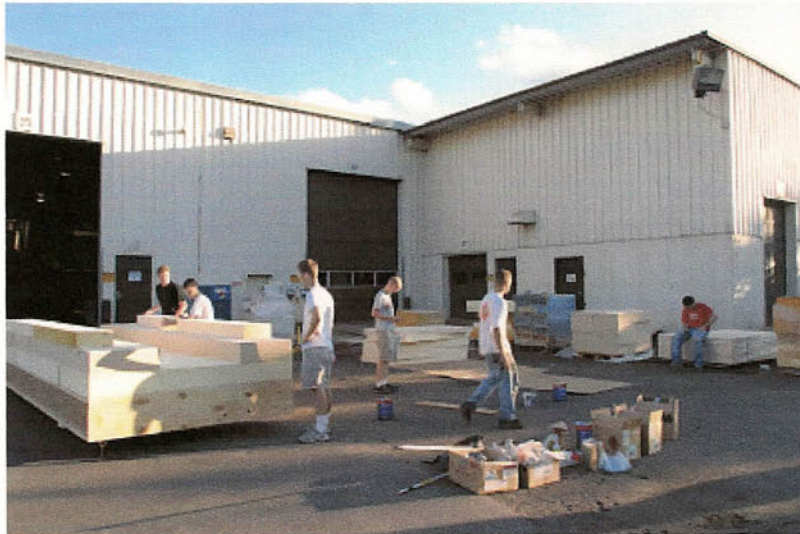
Figure 6: Foam Assembly onto Mold Bases at PaR
