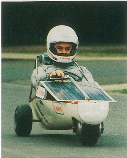
John Hill's "Dart", winner of the Electrokhana, has a small Solarex panel (0.675m 2 ) on a body that was once a kayak.
