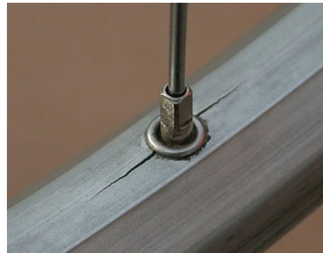
Figure 84 Rim spoke hole failure
