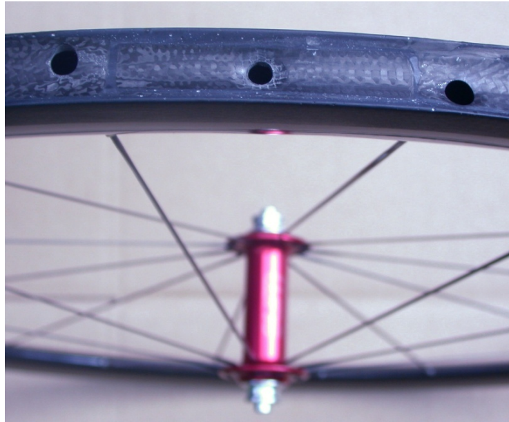
Figure 12 Carbon rim with angled spoke holes (type 1 stagger)
