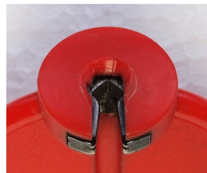
Figure 30 Modified jaws on the Spokey wrench
