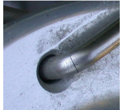
Figure 86 Spoke fatigue failure
