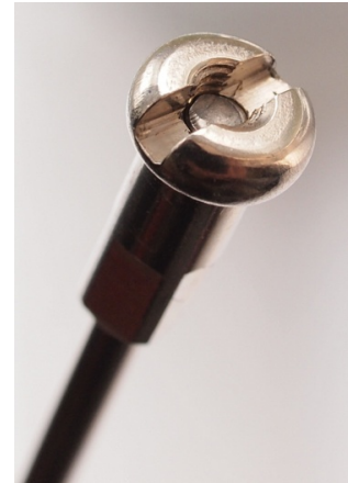
Figure 42 Position of the spoke in the measuring tool
