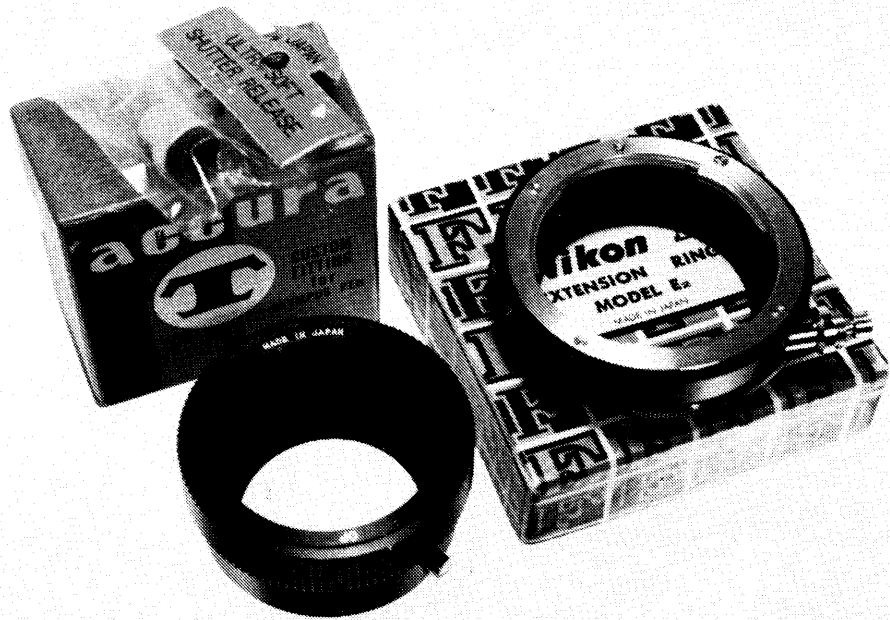
Materials for Nikon plunger adapter: Nikon E or E2 Extension Ring, Pen F T-mount, and soft shutter release accessory. Try finding them at places like Brooklyn Camera Exchange or Columbus Camera Group.
