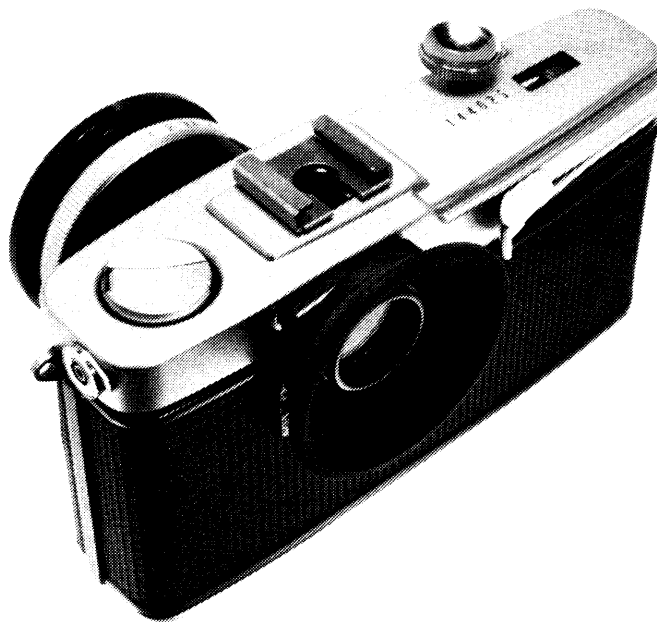
Finished eyecup adaptation on a modified Pen F Scientific Model, with soft shutter release in place and accessory shoe installed.
