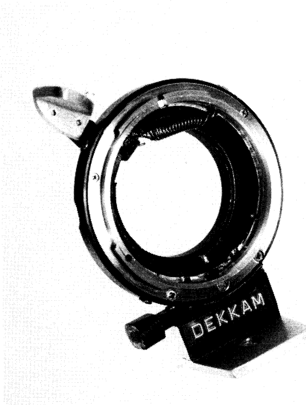
Canon lens to Pen F adapter by itself. The club-shaped protrusion near the bottom is the lever necessary to lock the adapter to the camera body, and is inset into a corner of the tripod support bracket.
