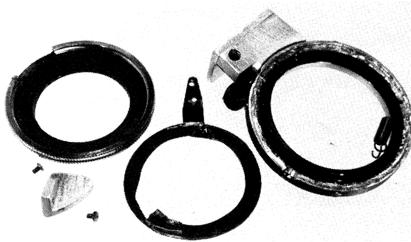
Parts of the Canon lens adapter. From top left, more or less clockwise: the short Pen F extension tube with part of its front circumference cut away to allow passage of the operating arm; the basic shell, made from a shortened Vivitar extension tube for the Canon FD mount, with spring anchored near the inner top; (center bottom) the actual operating lever, a circular piece of brass shim stock with an operating arm, a catch (just inboard of the arm, and hard to see since the whole part has been blackened) for the spring's other end, and a lug at the bottom to operate the lens' close-down lever; and the finger rest for the operating arm with its two retaining screws.
