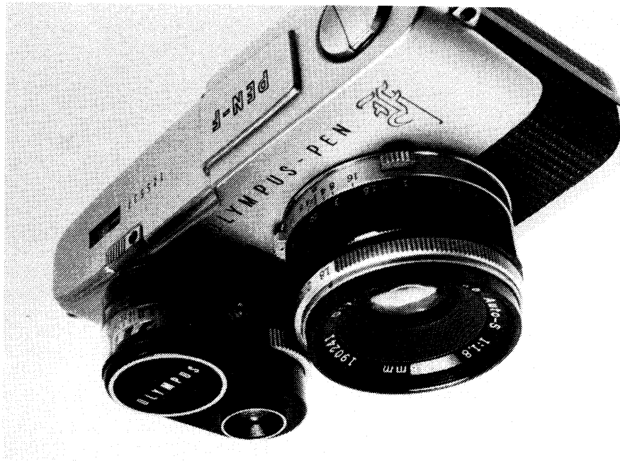
Accessory exposure meter mounted on the shutter dial of a Pen F. The "ASA Set" button is directly above the meter's embedded main setting wheel.
