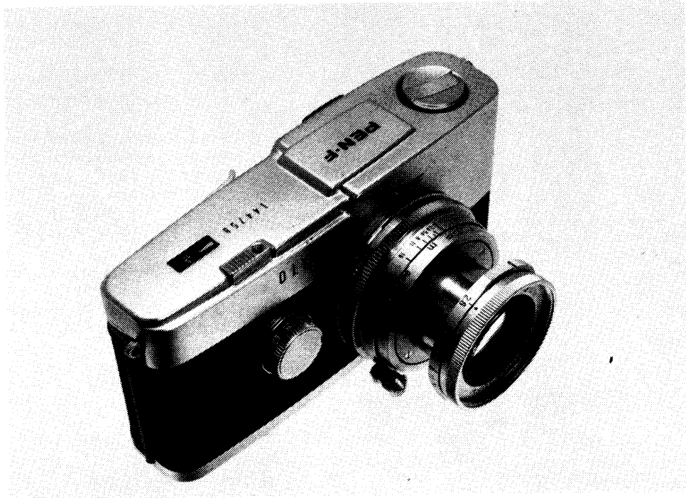
Pen FV with Leitz Elmar 50mm f/2.8 mounted via the Olympus Leica adapter; lens is not fully extended, as explained in the text.
