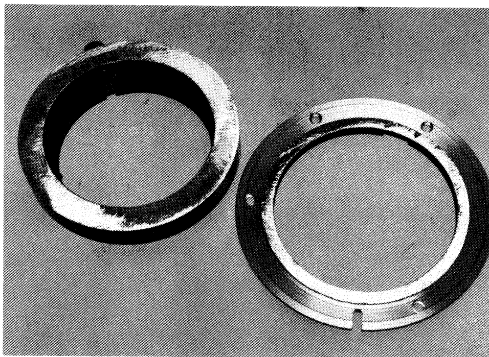
The modified parts: left, the Pen T-mount; right, the BR-4 flange with male Nikon bayonet removed. At this point about one millimeter of thickness remains to be cut away.
