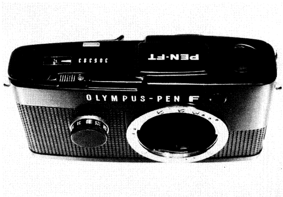
The Olympus Pen FT Scientific Model, with black insert in delayed action hole.
